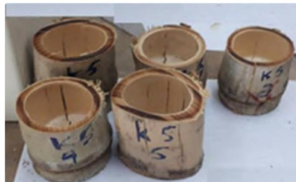
**Fig 3.** The compression test; (a) results; (b) specimens of Kara bamboo
