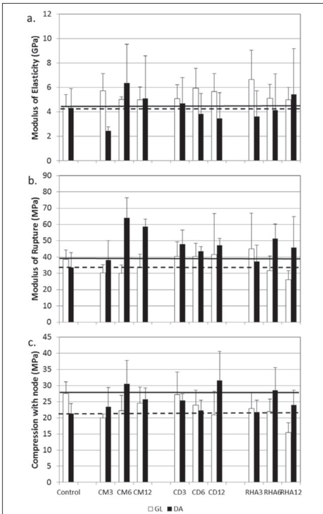
**Figure 1.** Mechanical properties of plantation-grown *Gigantochloa levis* and *Dendrocalamus asper* treated with organic fertilizers.
