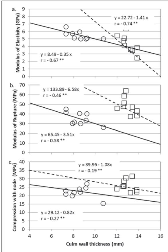
**Figure 4.** Effect of culm wall thickness on the mechanical properties of the culms. O = *Gigantochloa levis*; • = *Dendrocalamus asper*; \*\* = significant at 5% level; ns = not significant.
