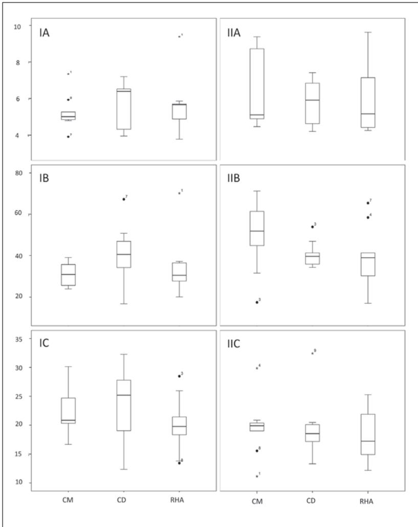
**Figure 2.** Influence of the organic fertilizer on the mechanical properties of the culms. I = *Gigantochloa levis*; II = *Dendrocalamus asper*; A = modulus of elasticity; B = modulus of rupture; C = maximum crushing strength.
