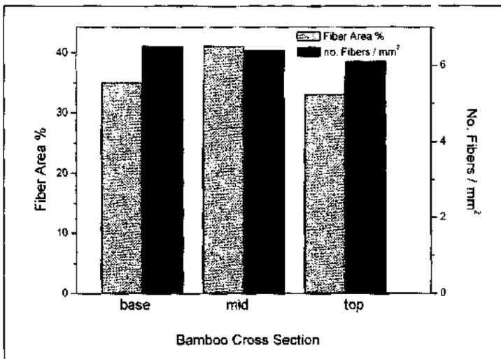
**Figure 6.** Percent area occupied by fibers and density of fibers (number of fibers per area) along the bamboo cross section.
