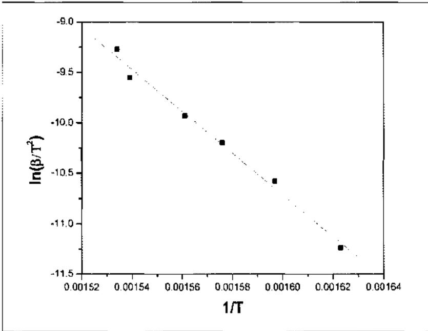
**Figure 3.** Plot of the experimental points using the Kissinger equation to evaluate the activation energy of the thermal decomposition process.
