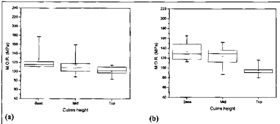
**Figure 8.** Variation of the modulus of rupture with the immersion time: (a) 10 days; (b) 54 days.
