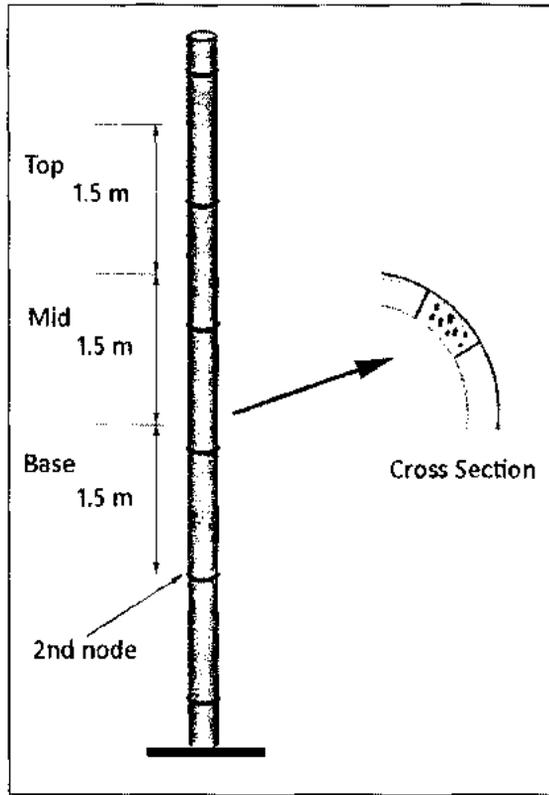
**Figure 1.** Distribution of the specimens along the height of the culms and orientation of the cross-section in relationship to the specimens' length.
