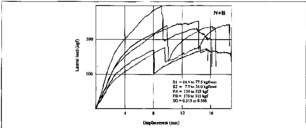
**Figure 8.** Lateral load-displacement characteristics of some screwed and bound (S+B) rattan joints.
