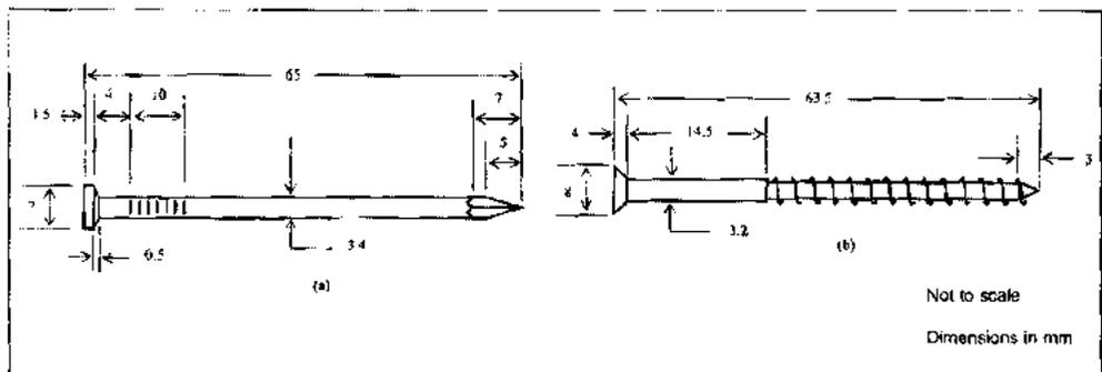
**Figure 3.** Nail (a) and screw (b) commonly used to fasten rattan furniture joints.
