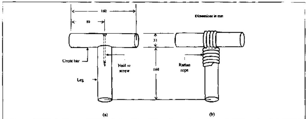
Figure 4. Rattan 'T' joint specimen (a) unbound (b) bound.
