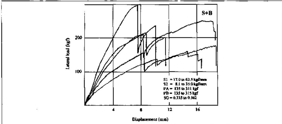
**Figure 9.** Lateral load-displacement characteristics of some screwed and bound (S+B) rattan joints.
