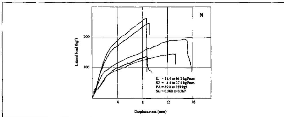
Figure 6. Lateral load-displacement characteristics of some screwed (S) rattan joints.
