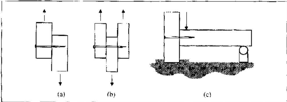
**Figure 2.** Lateral load test: (a) single shear, (b) double shear, (c) 'T' joint.
