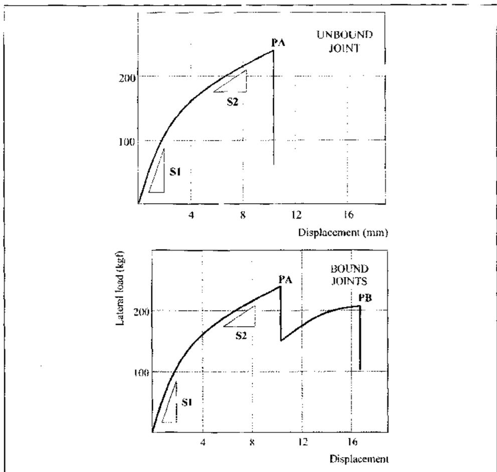
Figure 5. Lateral load-displacement characteristics of some nailed (N) rattan joints; S1: Slope 1; S2: Slope 2; PA: Peak A; PB: Peak B; SG: Specific gravity.
