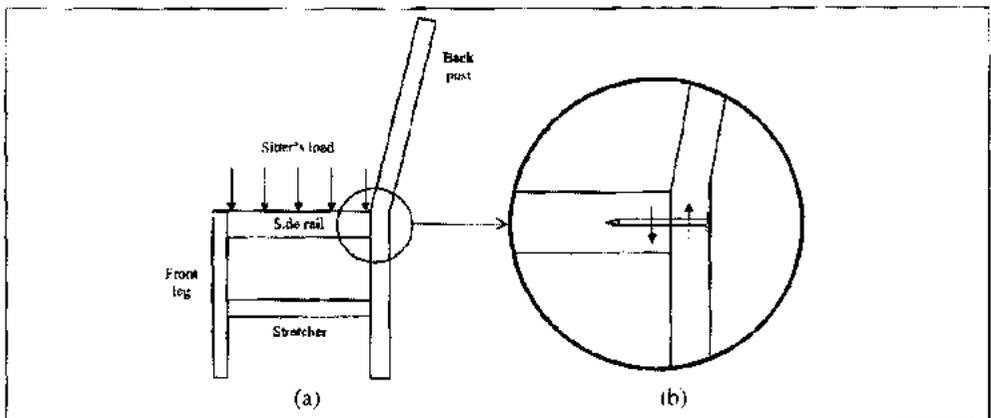
**Figure 1.** Typical chair side frame: (a) under sitter's load, (b) lateral loading effect at the side rail to backpost.
