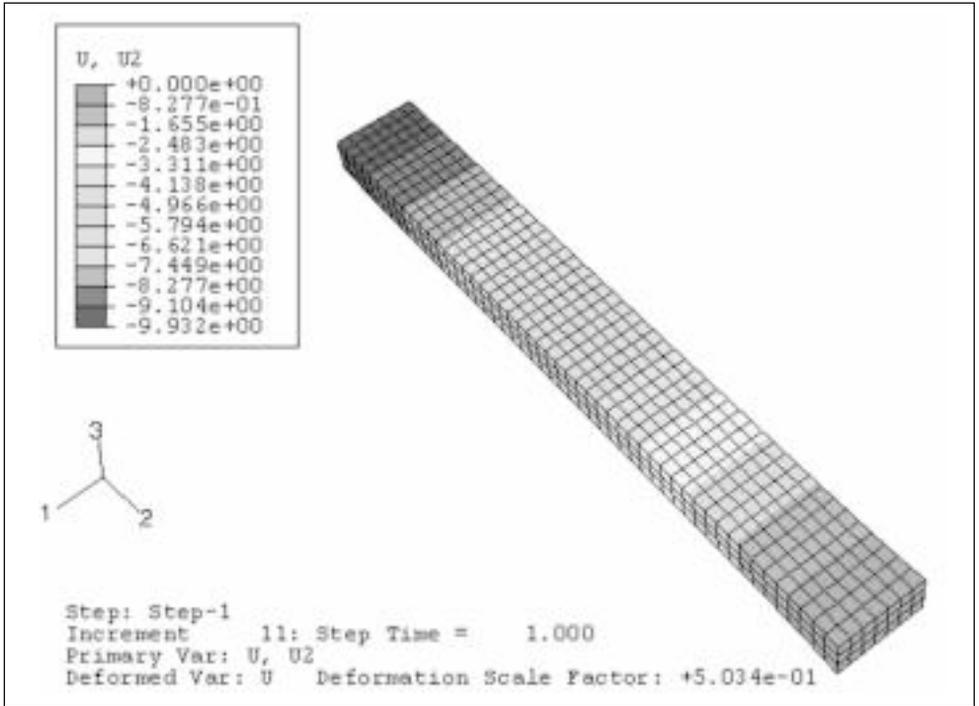
Figure 2. Deflection contour plot for the outermost sample.
