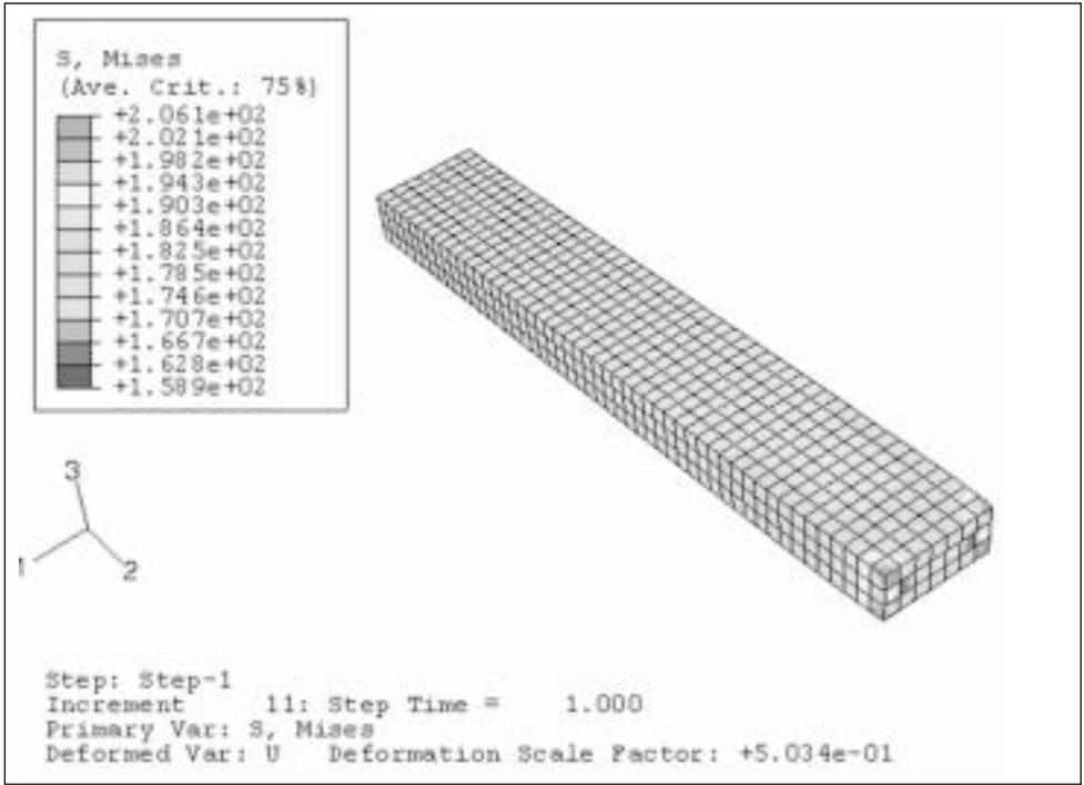
**Figure 4.** Mises stress contour plot for the outermost sample.
