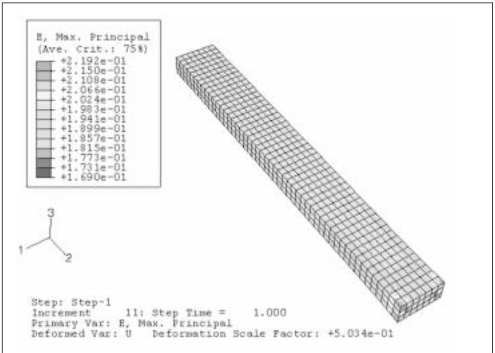
Figure 3. Strain contour plot for the outermost sample.
