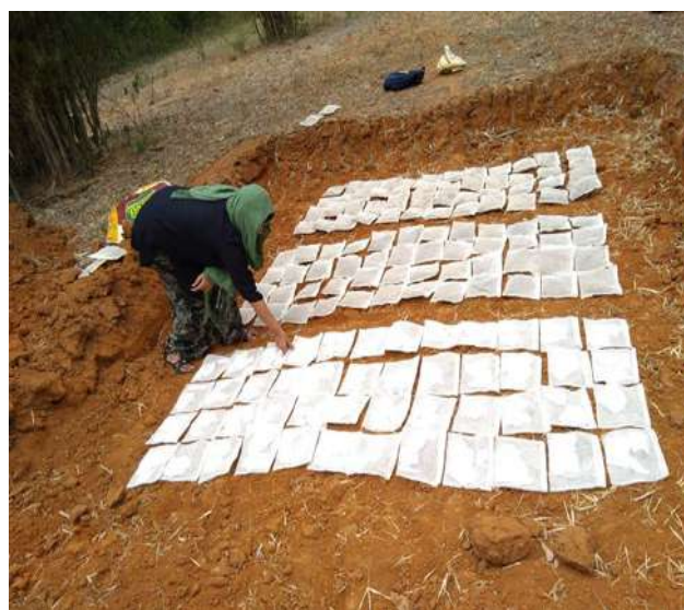
Fig 2 . Sub-surface placement of litter, twig and filter paper samples for decomposition experiment
