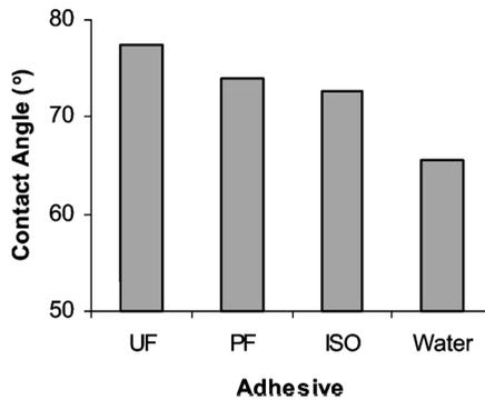
**Figure 1.** Effects of four adhesives (UF, PF, ISO and distilled water) on the mean contact angle of Honduran bamboo.
