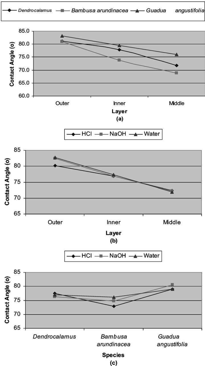
**Figure 2.** Interaction between layer and species, layer and chemical treatment, and species and chemical treatment of the contact angle of UF resin.
