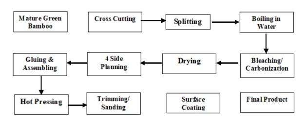
Fig 2. Flow chart for the manufacture of bamboo wood
