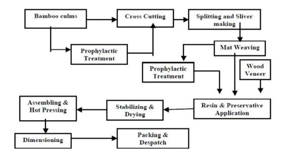
Fig. 1. A generalized process flow chart for Bamboo Mat Composites
