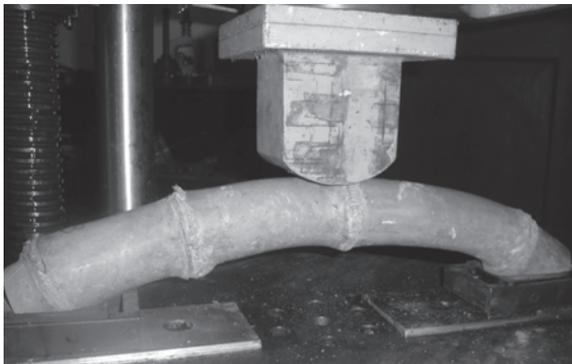
**Figure 2.** Mechanical test on one of the culturally preformed *Bayog* specimens, using three-point loading due to the short span of the test samples. Grease was applied between the contact points of the support and the ends of the preformed bamboo.
