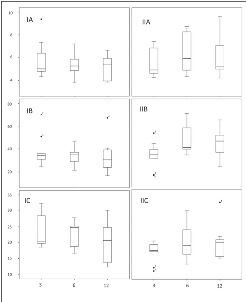
**Figure 3.** Influence of the rate of fertilizer application on the mechanical properties of the culms. I = *Gigantochloa levis*; II = *Dendrocalamus asper*; A = modulus of elasticity; B = modulus of rupture; C = maximum crushing strength.
