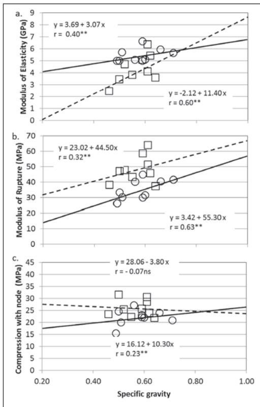
**Figure 5.** Effect of specific gravity on the mechanical properties of the culms. O = *Gigantochloa levis*; • = *Dendrocalamus asper*; \*\* = significant at 5% level; ns = not significant.
