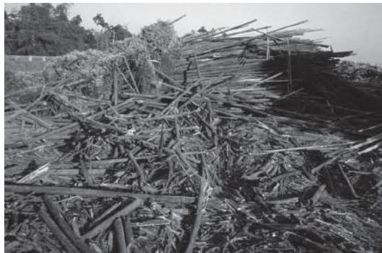
Figure 8. Fungal deterioration of a bamboo pile at a pulp mill.
