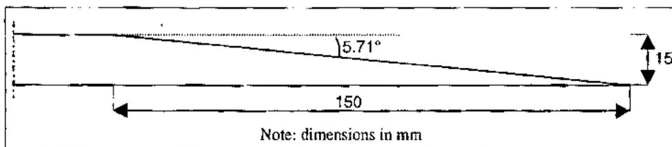
**Figure 4.** Scarf joint geometry
