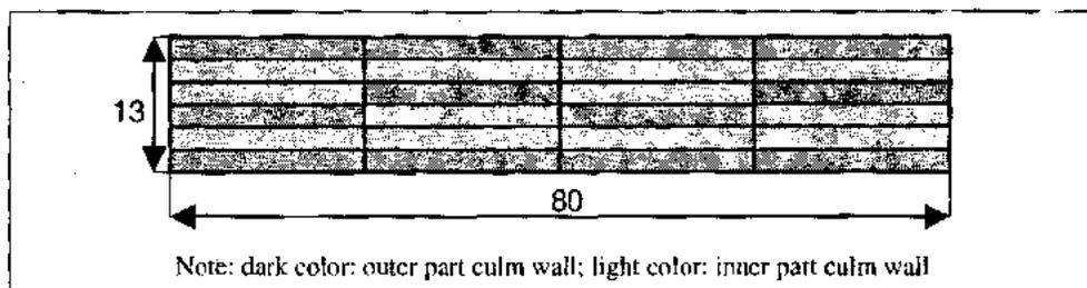
Figure 2. Composition of three-layer laminations
