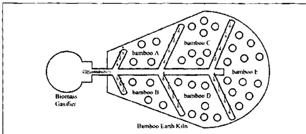
**Figure 4.** Integration of a bamboo carbonisation kiln with a biomass gasifier.
