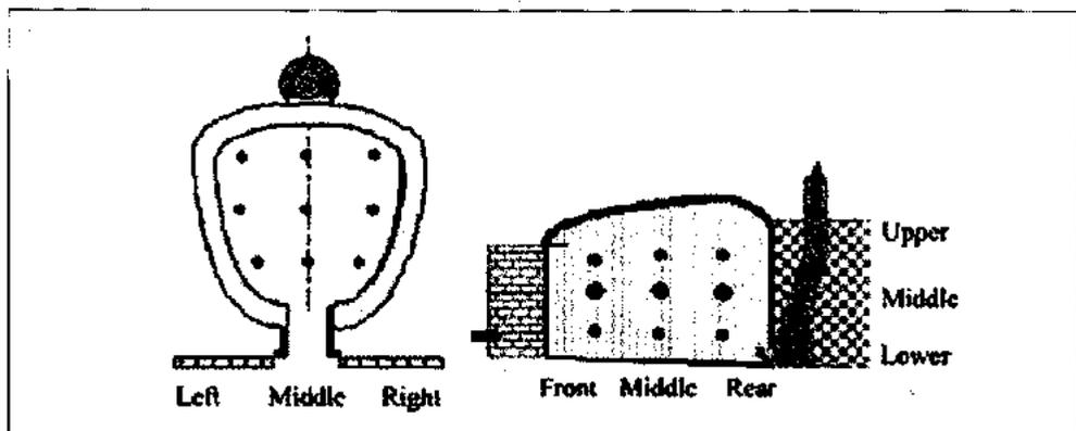
Figure 5. Kiln temperature monitoring layout.
