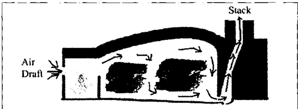
Figure 1. Schematic diagram of a Japanese Schwartz type Earth Mound Kiln.
