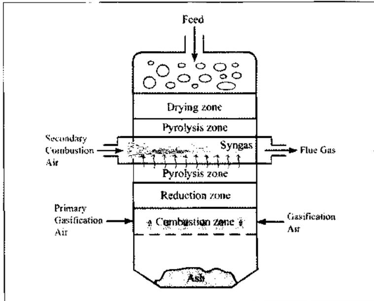
**Figure 2.** The schematic diagram of the modified fixed bed gasifier.
