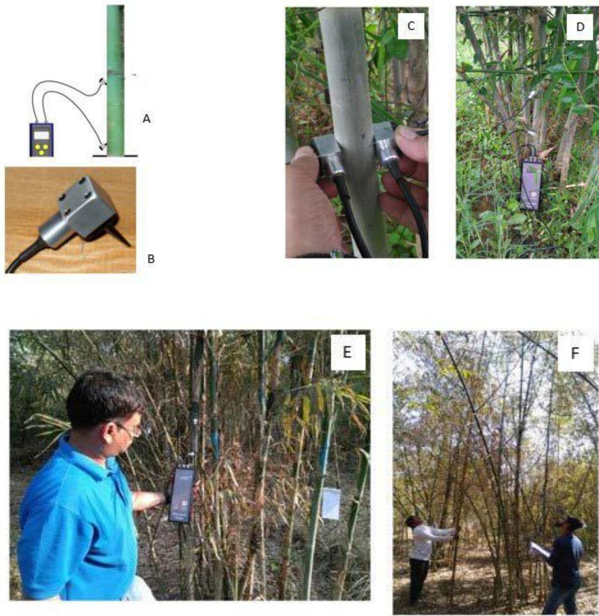
**Fig 2.** Ultrasonic measurement and field data collection (A- scheme of ultrasonic measurement, B- probes used for measurement, C- measurement for hollowness, D – along the length measurement of ultrasonic velocity, E- Ultrasonic data recording, F- culm assessment)
