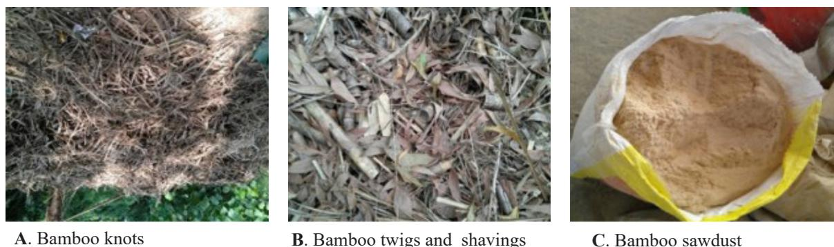
**Figure 4:** Waste generated during the bamboo cutting and splitting
