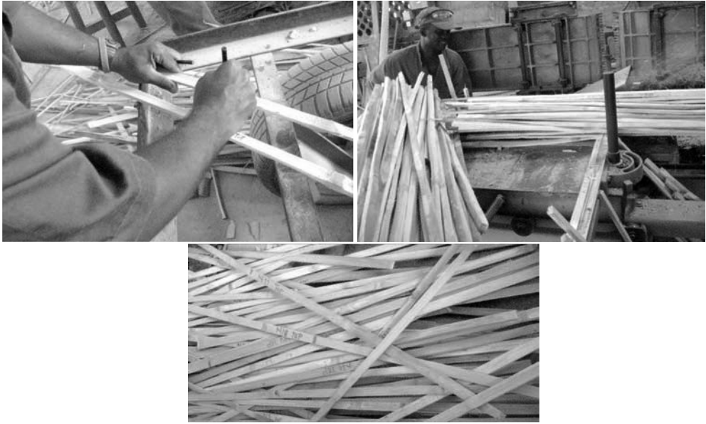
Figure 4: Bamboo strips being planed and labeled
