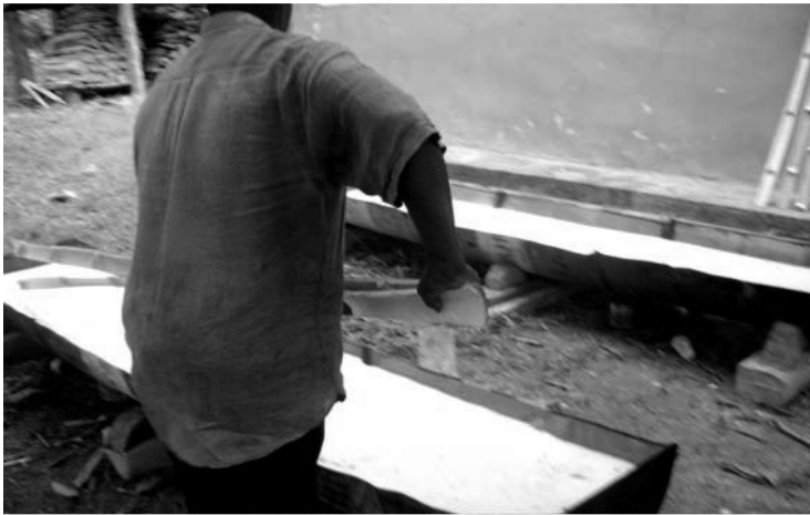
Figure 2: Chemical treatment of bamboo strips through dipping method
