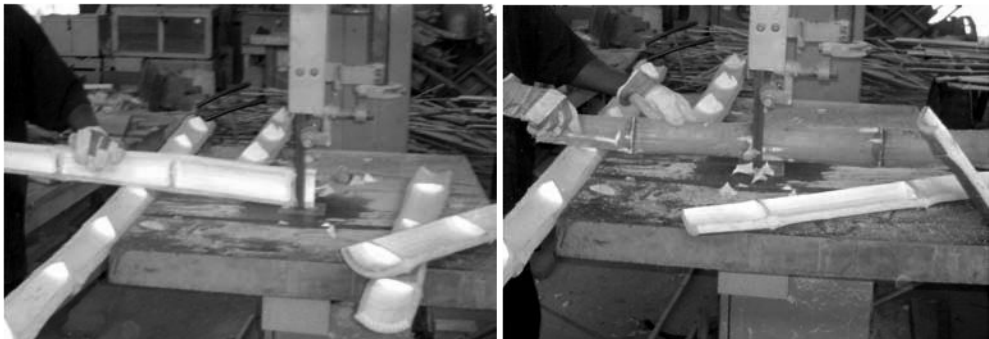
Figure 3: Removal of diaphragms and other knots from bamboo strips
