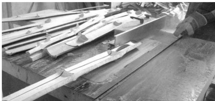
Figure 1: Ripping and re-ripping of bamboo culms with Arbor saw-bench
