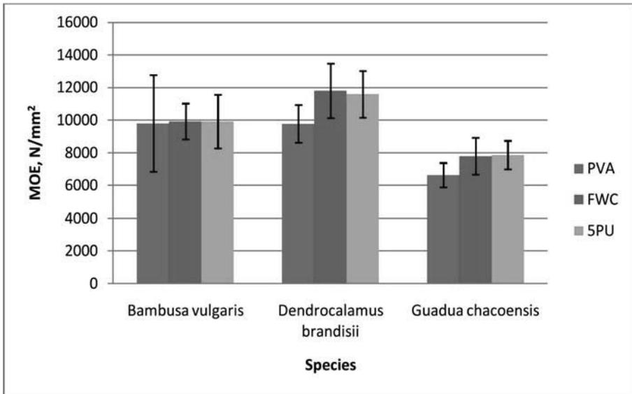
Figure 2: Modulus of Elasticity (MOE) of the species for each glue type
