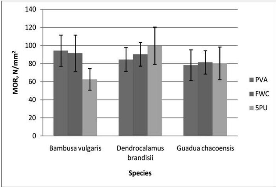
Figure 1: Chart showing the Modulus of Rupture (MOR) of the species for each glue type
