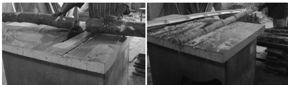
Figure 2: A- Cross-cutting & B- Ripping of bamboo culms with wood processing machine
