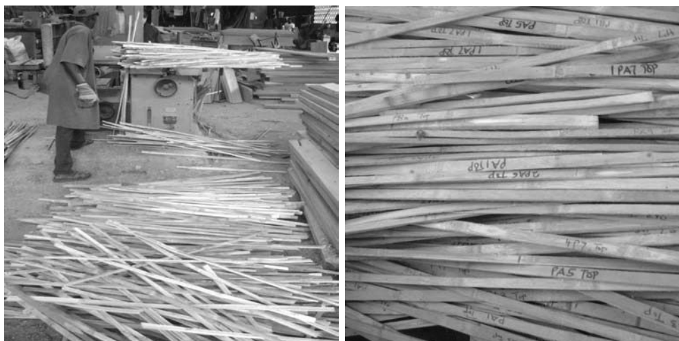
Figure 5: A-Planing of bamboo strips with a thicknesser machine, B- Planed bamboo strips
