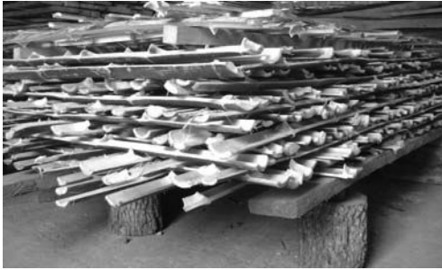
Figure 3: Treated Bamboo strips stacked for air-drying
